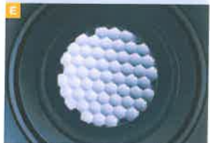
Fly-eye lens for homogeneous fluorescence illumination
