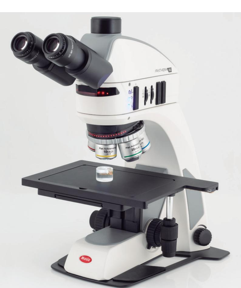
Smart Darkfield with 5 Segment illumination mode New LD Plan Achromatic and S-Apochromatic BD objectives & 22mm FOV eyepieces Pure incident or incident/ transmitted microscope stands available
