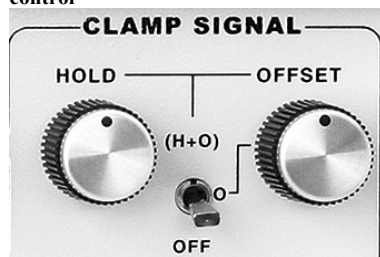
Figure 31. Hold and Offset command control
