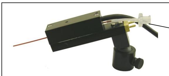
The input of the HCPC is silicone tube equipped with a female Luer connection. The ID of the silicone tube is about 1mm so most ALA manifolds can be connected directly to the tubing if the Luer is removed. Otherwise your perfusion system can be coupled to the HCPC with a male Luer.
