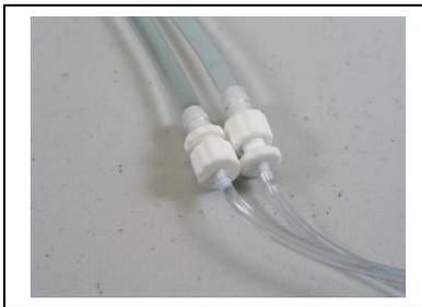
Two Luer fittings shown at left connect the cooler to the HCPC. When the HCPC is to be disconnected, connect the Luer fittings together to form a loop (right) so the fluid does not leak out. When connecting/disconnecting tubes always keep the connections 0.5-1M above the cooler to keep a siphon that will keep the liquid from leaking out during the process.
