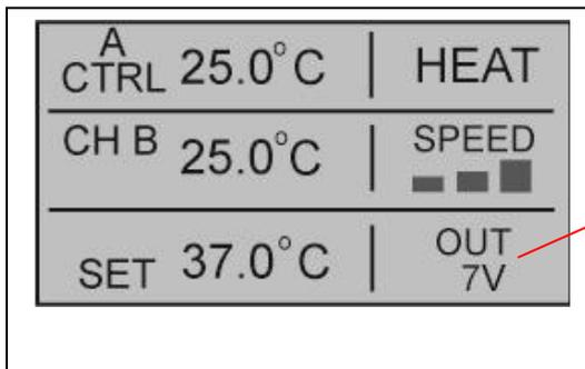
To limit the power on the HCT from ALA, set the voltage output to 7 volts.
