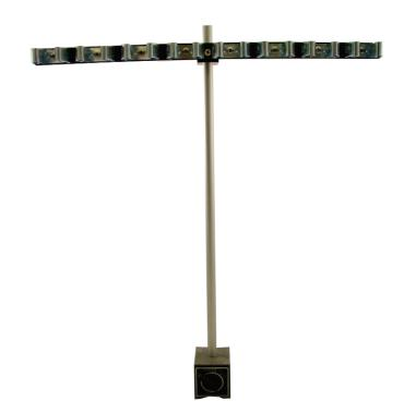
Set up stand as shown in bottom image. Each 60ml reservoir will snap into the clips attached to the bracket.
