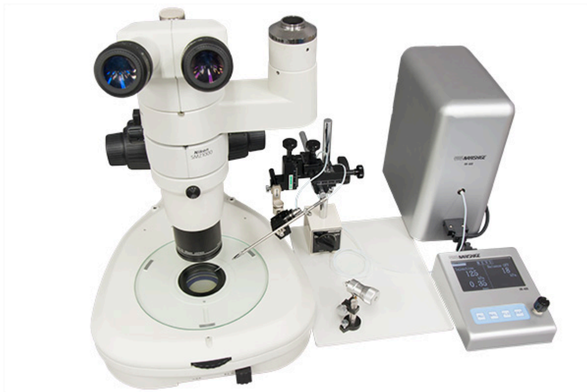
DNA injection set ( IM-400 + MMO-220C + M-152 + GJ-1 + IP )
