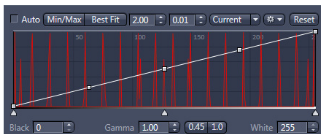
Gamma adjustment – linear display
