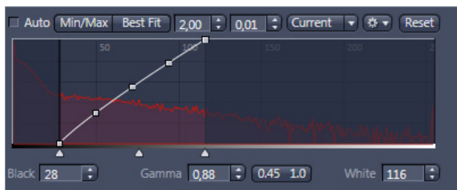
The same image displayed with a steep display curve – cutting away some of the dark and bright information – shows too much contrast.
